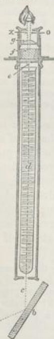
Plan of the Apparatus for showing the circular polarisation of liquids. In this figure, g indicates a lens which is used to produce well-defined images.
